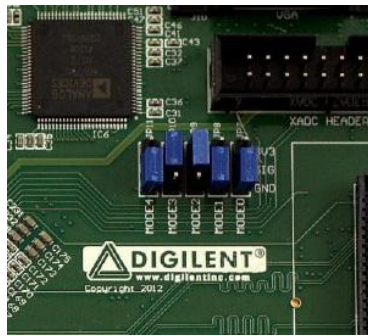
Figure 16: ZedBoard SD Card Boot Mode Jumper Setting
