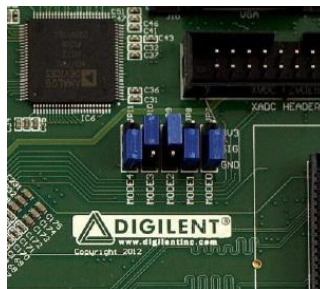
Figure 167: ZedBoard SD Card Boot Mode Jumper Setting
