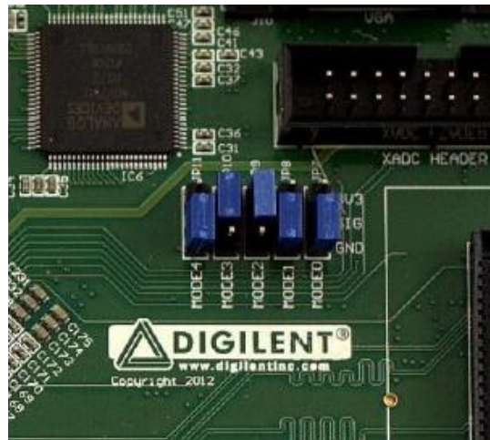
Figure 97: ZedBoard SD Card Boot Mode Jumper Setting
