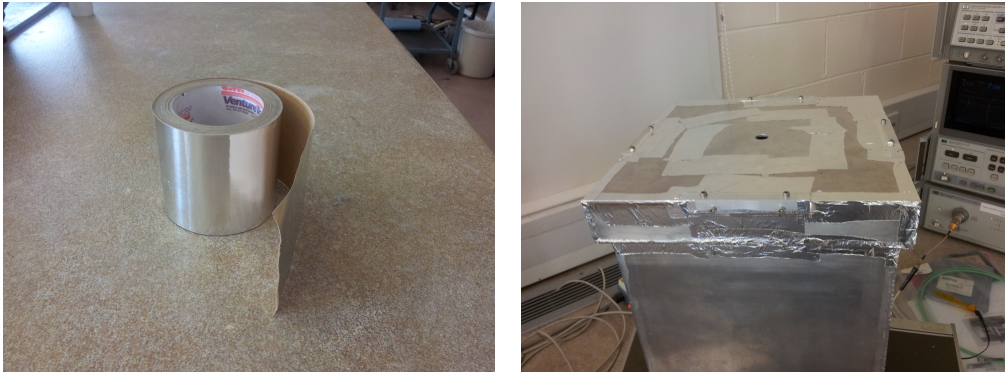
Figure 5.11: Applicator covered with metal tape.
