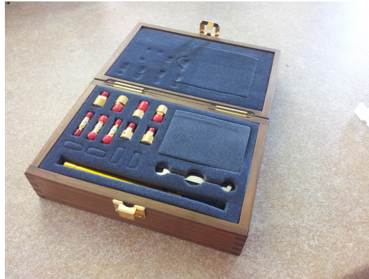
Figure 5.10: Calibration kit for the VNA.
