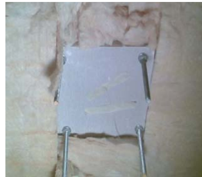
Figure 4 Experimental setup. 18 SmartBoards bolted together and surrounded by insulation.
