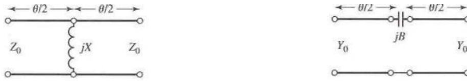
Figure 2.17: Shunt inductance equivalent circuit for an impedance inverter. Figure 2.18: Series capacitance equivalent circuit for an admittance inverter.
