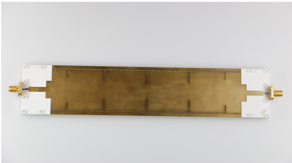
Figure 5.12: Final filter that has been manufactured with \epsilon_r modified
