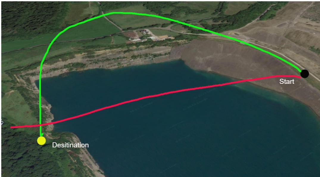
Figure 5.1: A drone travels from the start to the destination, crossing a lake. Features detected on the water surface are not consistently tracked, hence negatively impacting the VO performance. The red trajectory, despite being shorter, lacks reliable visual features for pose tracking. In contrast, the longer green trajectory enhances visual odometry performance by maximising reliable feature quality over terrain, houses, etc.
