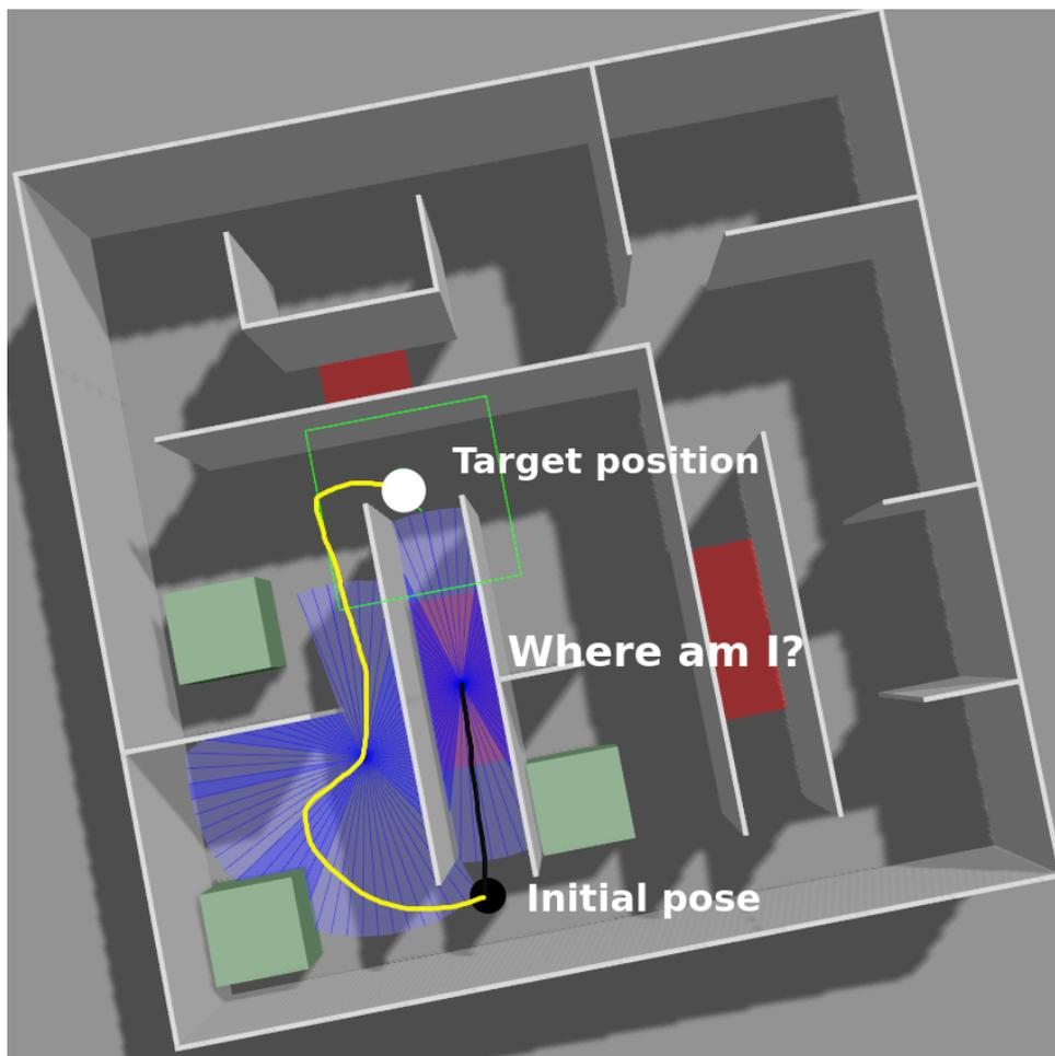
Figure 4.3: Navigation examples (red regions: regions where localisation fails; black trajectory: unsuccessful trajectory into the symmetric corridor; yellow trajectory: successful trajectory avoiding the symmetric corridor.)
