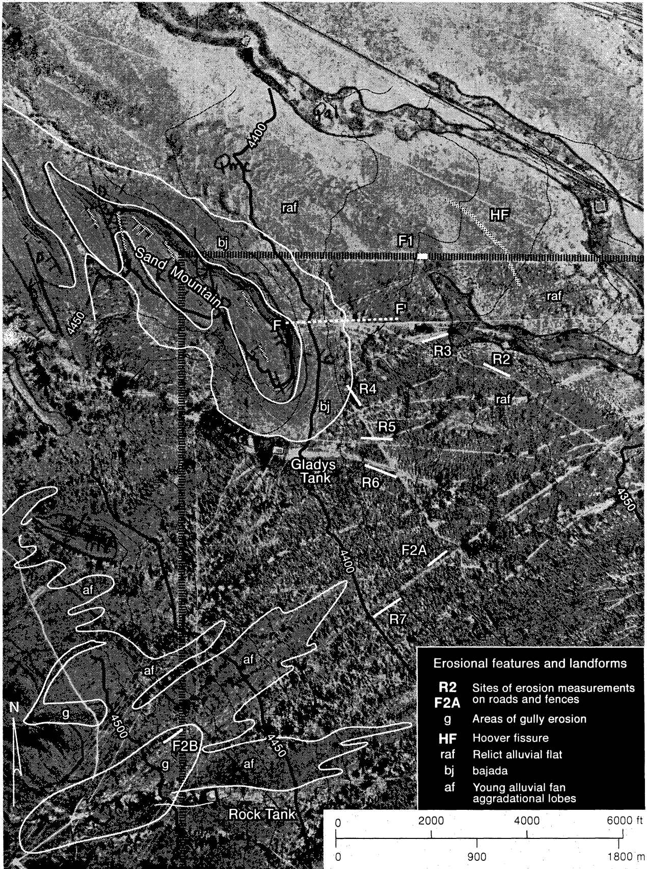
Figure 13. Aerial photograph of Sand Mountain area with topographic contours and locations of selected landforms and erosional features. The sites of erosional measurements of roads (R2 through R8) and fences (F1, F2a, F2b) are numbered as they are in table 5. F-F' shows the location of figure 14. Location shown in figure 4.
