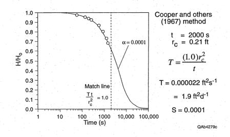
Figure 10. Results of a bail test at CBW-B002.
