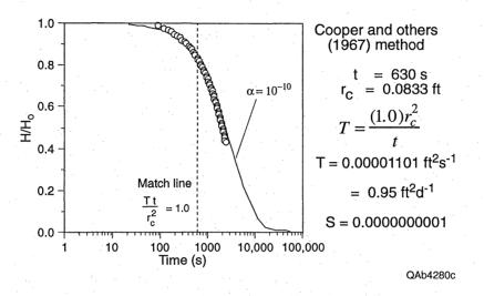
Figure 11. Results of a bail test at CBW-B013.
