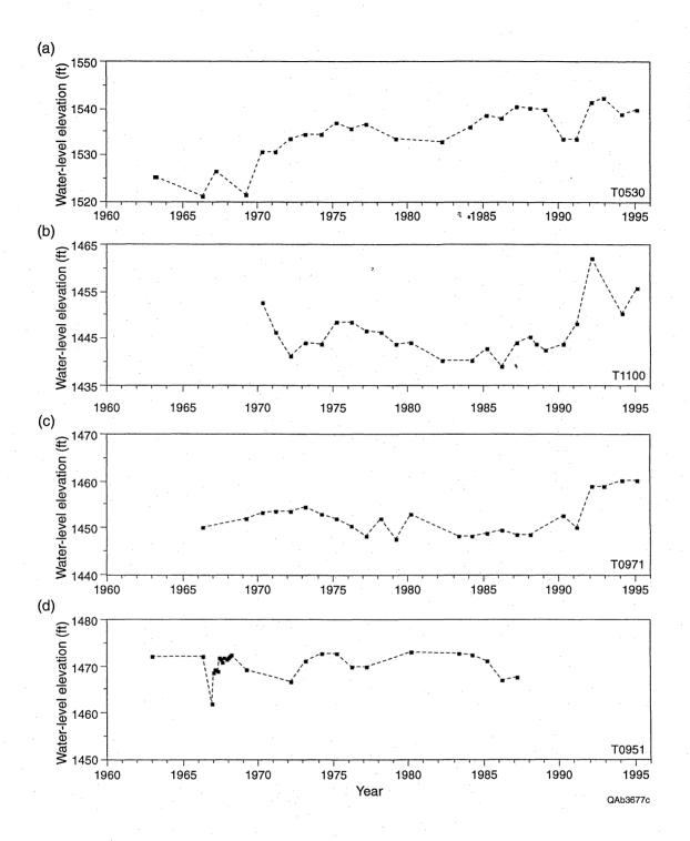
Figure 5. Water levels measured in Travis Peak Formation for wells (a) 41-09-303, (b) 41-18-650, (c) 41-18-303, and (d) 41-18-205 in Brown County.
