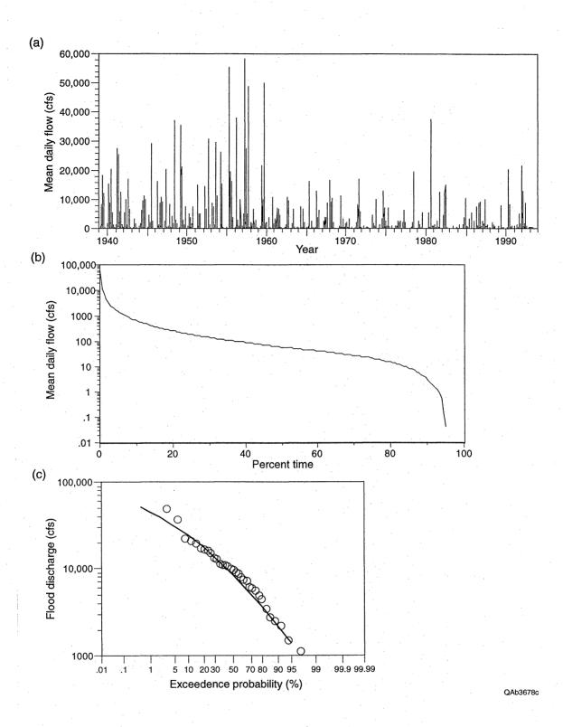
Figure 17. (a) Mean daily flow, (b) flow duration, and (c) flood frequency analysis using a Log Pearson III fit for a stream gauge in the Colorado River near Winchell.
