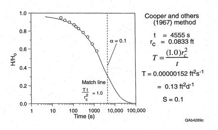
Figure 9. Results of a bail test at BOWIE-2.
