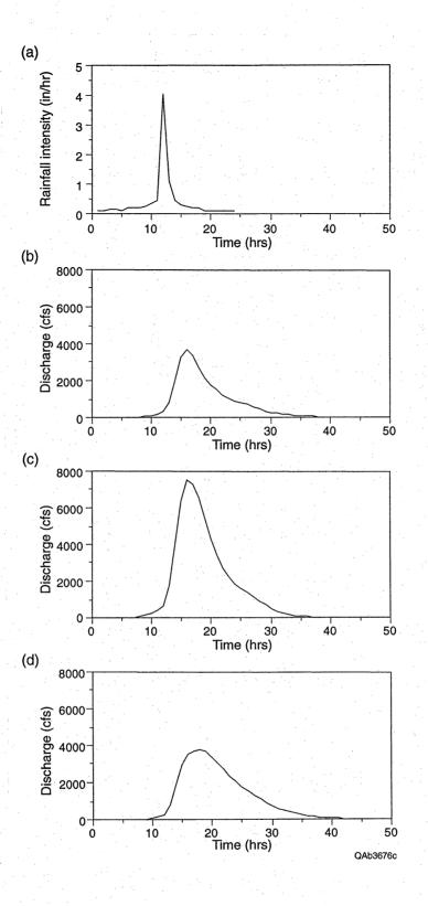
Figure 19. Flood hydrograph analysis of Camp Bowie: (a) 100-yr 24-hr SCS Type II distributed rainfall intensity and the 100-yr flood hydrographs near the camp boundary of (b) a tributary to Mackinally Creek (point A, fig. 15), (c) Devils River (point B, fig. 15), and (d) Lewis Creek (point C, fig. 15).
