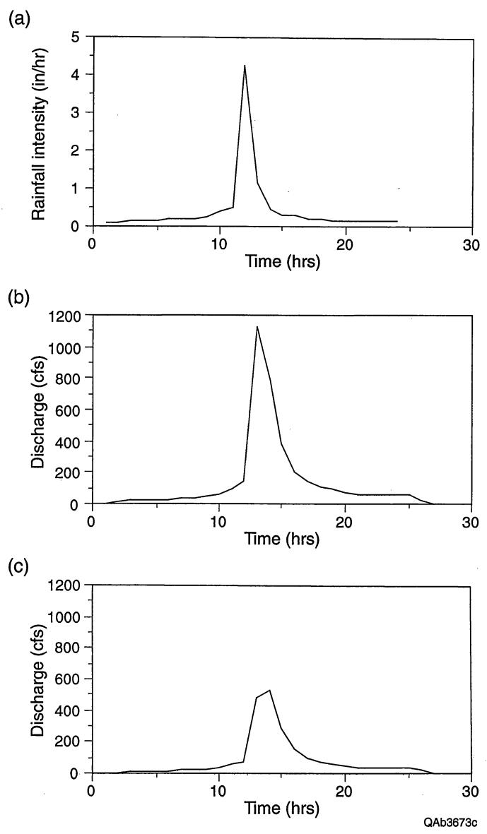
Figure 17. Flood hydrograph analysis of Camp Mabry, including (a) 100-yr 24-hr SCS Type II distributed rainfall intensity and 100-yr flood hydrographs near the camp boundary for the (b) eastern stream (point A, fig. 15) and (c) western stream (point B, fig. 15).
