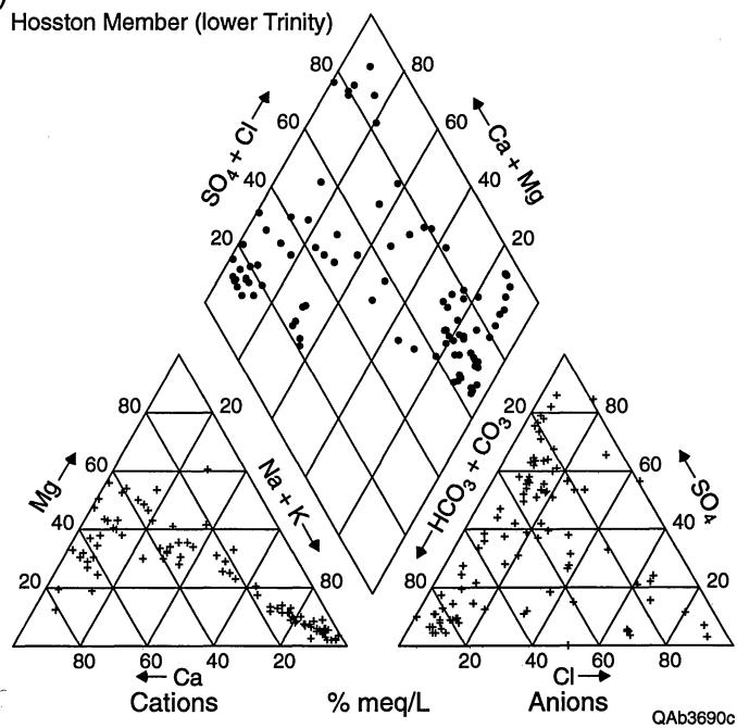
Figure 14. Trilinear diagram showing chemical composition of ground-water samples from the (a) Glen Rose Formation and (b) Hosston Member of the Travis Peak Formation (Lower Trinity) in Travis County.
