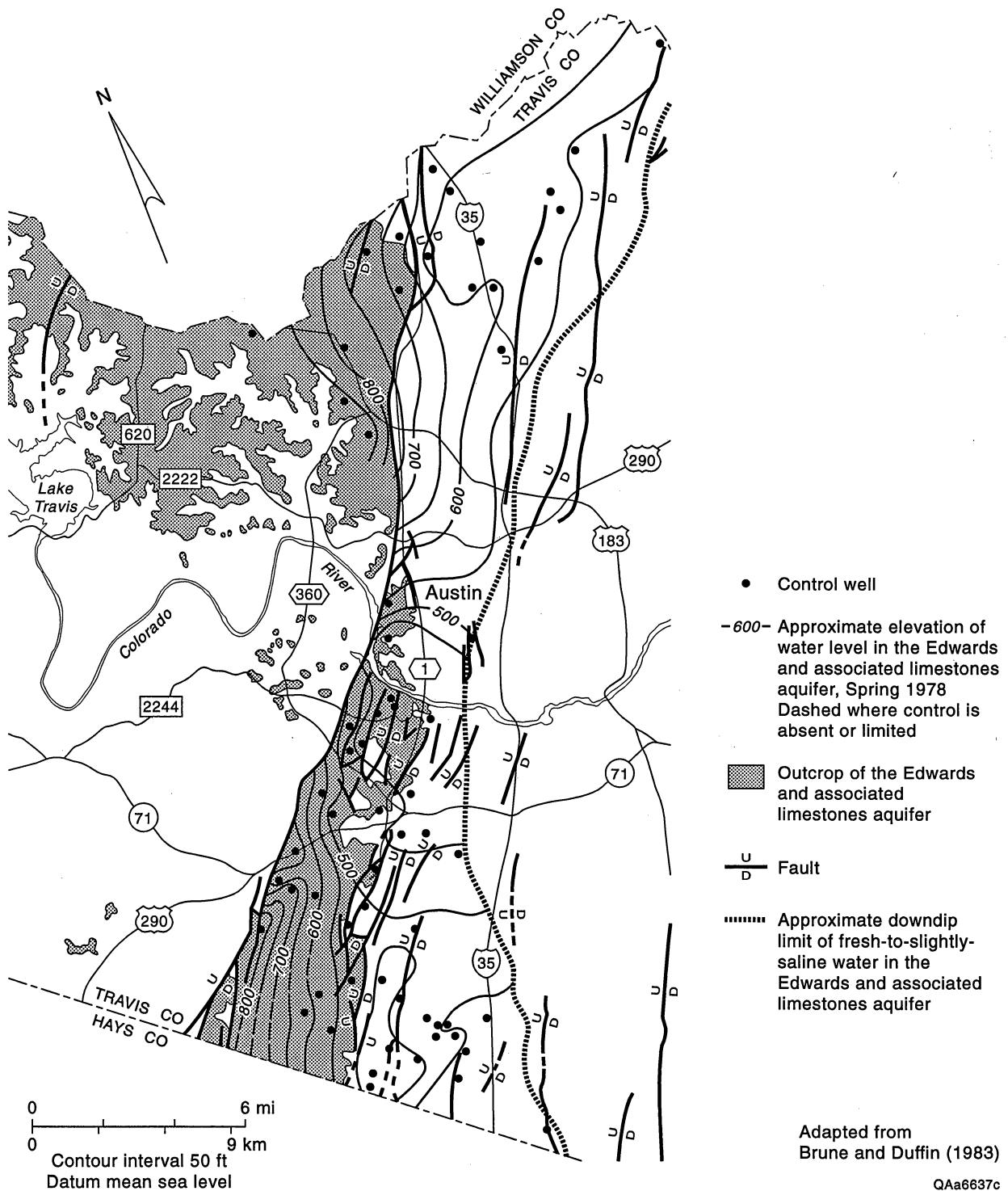
Figure 7. Approximate altitude of water levels in wells completed in the Edwards and associated limestones aquifer, spring 1978, from Brune and Duffin (1983).
