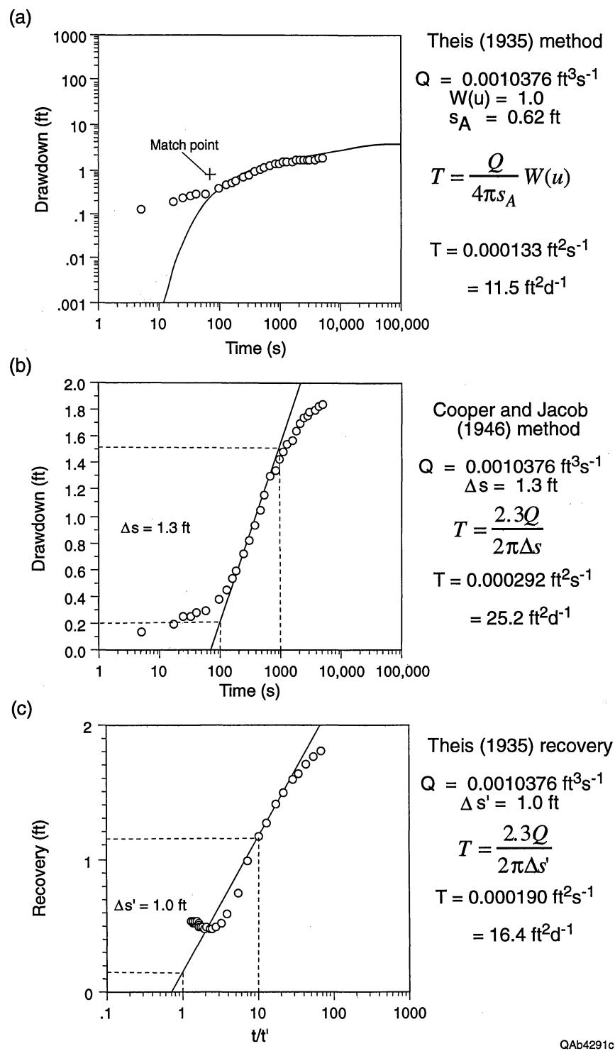
Figure 10. Results of a pumping test in the upper part (fill) of MABRY-1.
