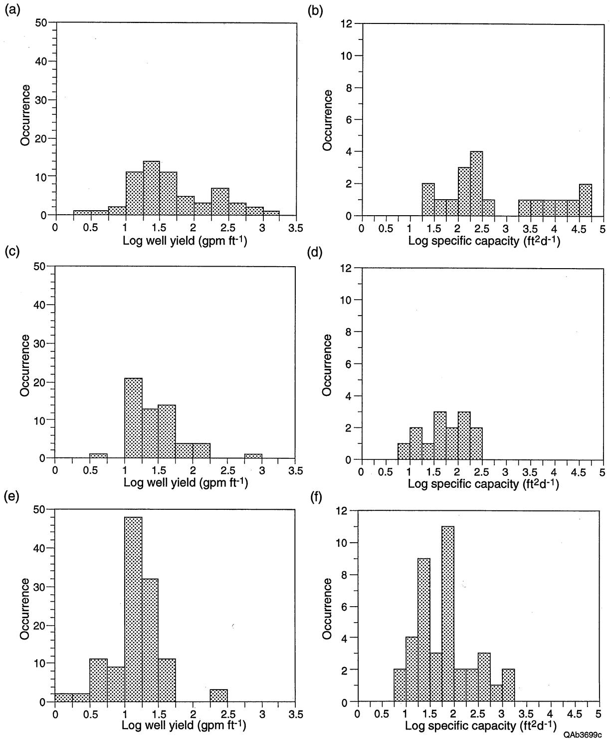
Figure 9. Well yields and specific capacity of the Edwards and associated limestones (a, b), the Lower Trinity (c, d), and the Glen Rose Formation (e, f).
