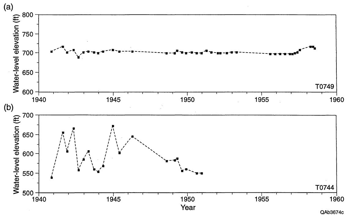
Figure 6. Water levels measured in Travis County in the Austin Chalk in (a) well 58-43-502 and (b) well 58-43-402. Well 58-43-502 is shallow (40 ft deep) and probably completed in weathered chalk, whereas well 58-43-402 is deeper (184 ft deep) and, because of its large variations in water level, probably intersects a fault zone. These two wells are 0.3 mi apart.
