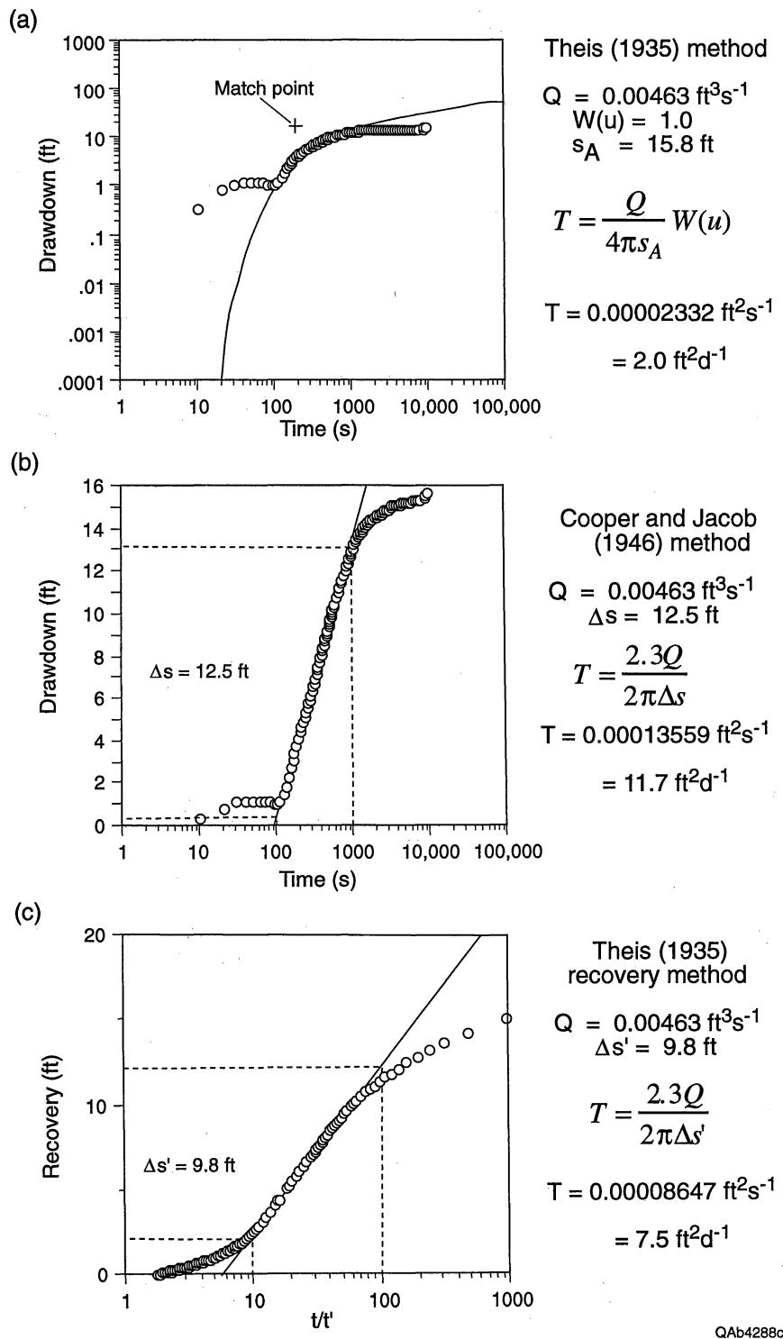
Figure 11. Results of a pumping test in the lower part (Edwards) of MABRY-1.
