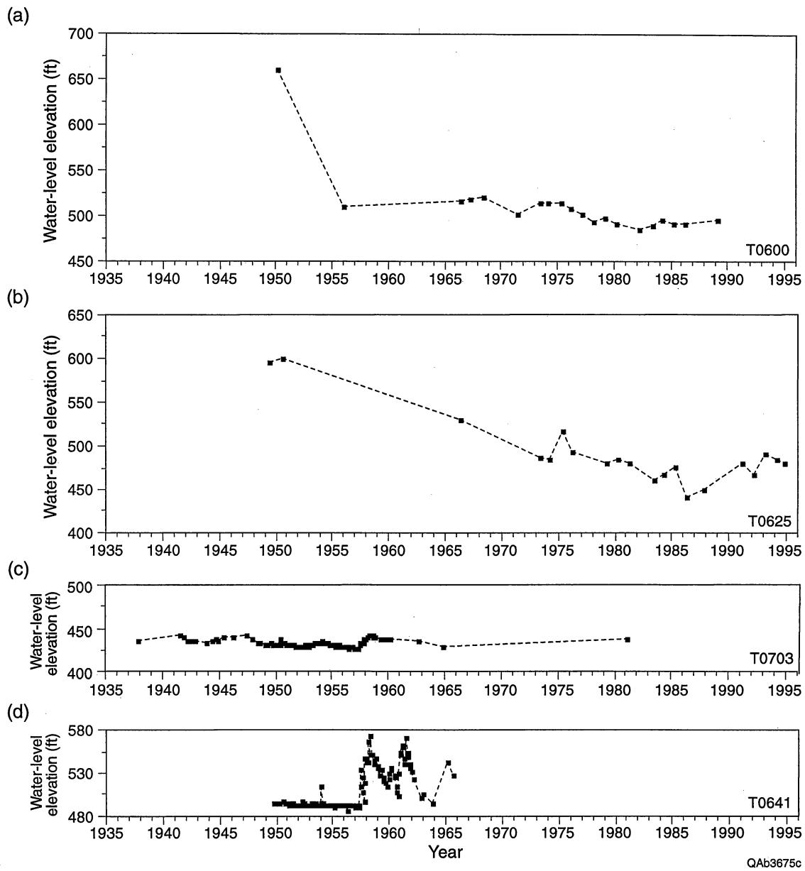
Figure 5. Water levels measured in Travis County in the Hosston Member in (a) well 58-42-302 and (b) well 58-42-502 and in the Edwards Formation and associated limestones in (c) well 58-42-911 and (d) well 58-42-602.
