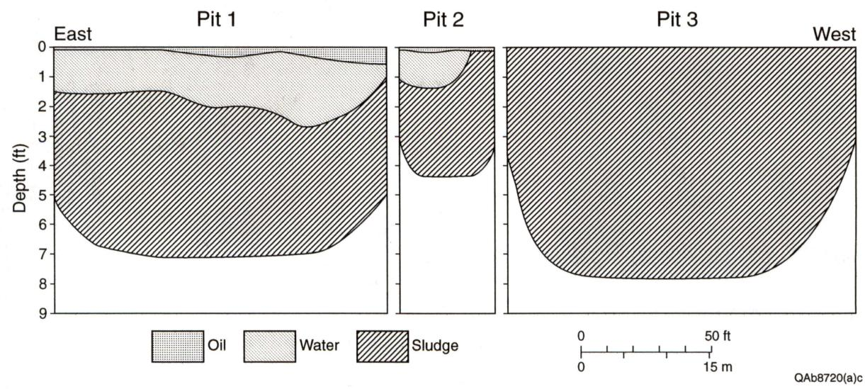
Figure 3. Profile of pit-fluid layers.
