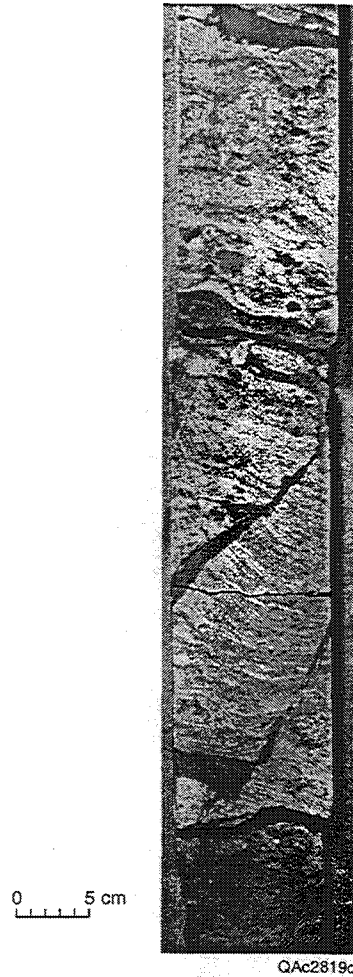
Figure 27 (cont.). Breccia interpreted as a result of formation and collapse of natural salt caverns. (b) Open fractures and rotated blocks above a large collapsed salt cavern, DOE Stone and Webster Sawyer core, 674 ft below datum.
