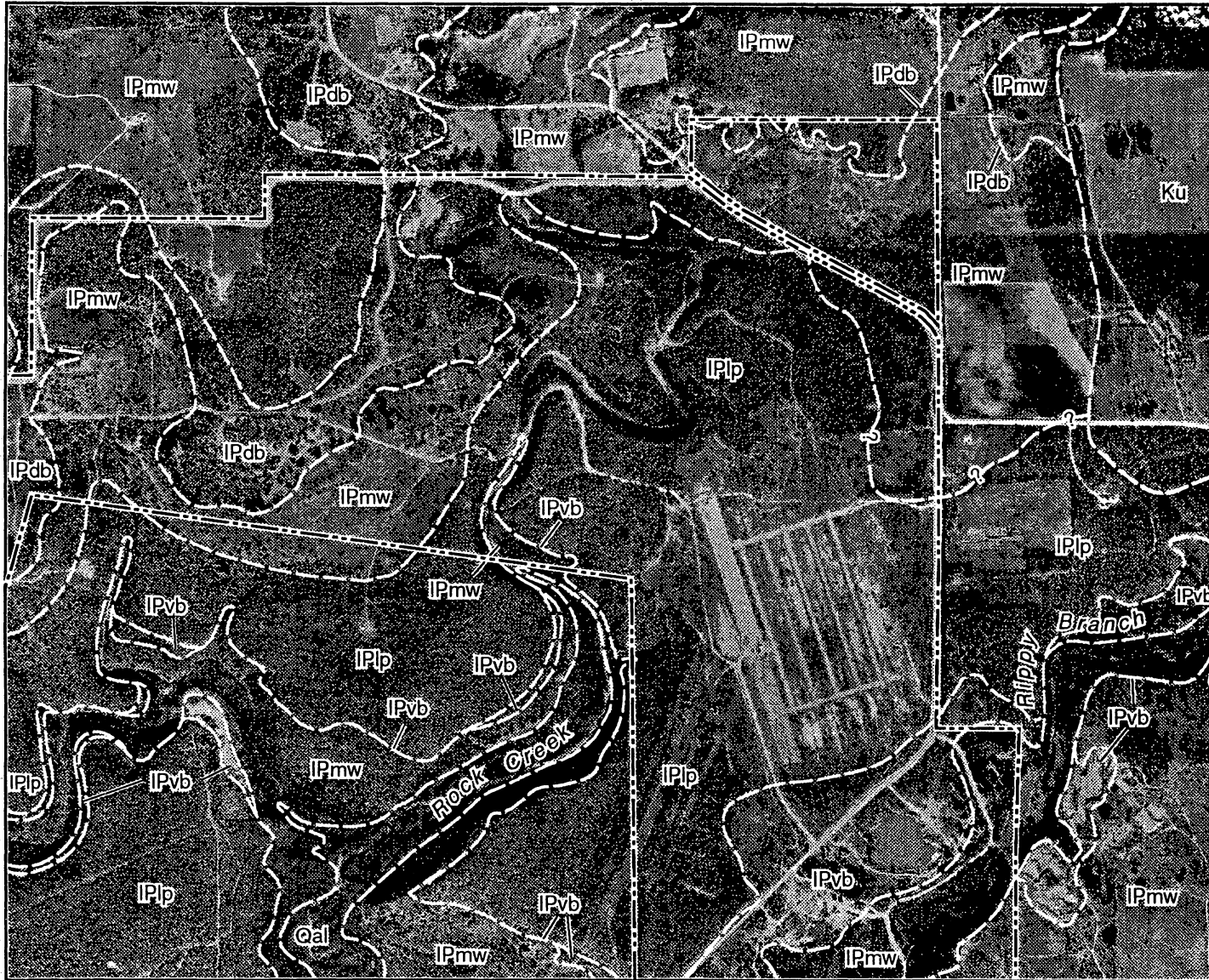
Figure 8b. Geologic map of northeast portion of Fort Wolters on unrectified aerial photograph base (NAPP 2342-68; see table 1); see figure 8a for explanation of map symbols.
