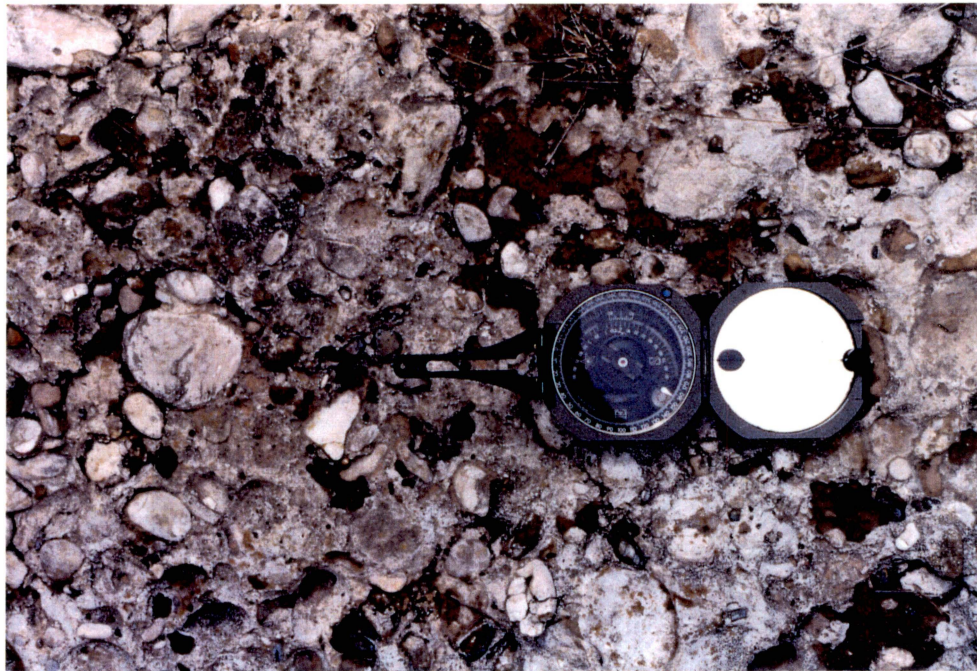
Figure 9. Photograph of well-cemented pebble conglomerate at base of Travis Peak Formation. Compass 2.75 inches in diameter.
