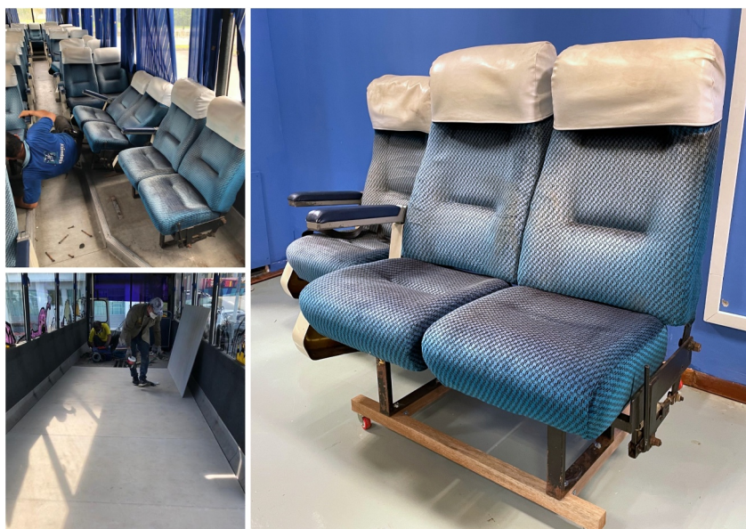
FIGURE 6 Before and after: The original bus seats were repurposed as moveable seating for use in the CreativeCulture lab. Seat pairs were augmented with wooden bases, complete with castors, to allow for easy movement within the space.
