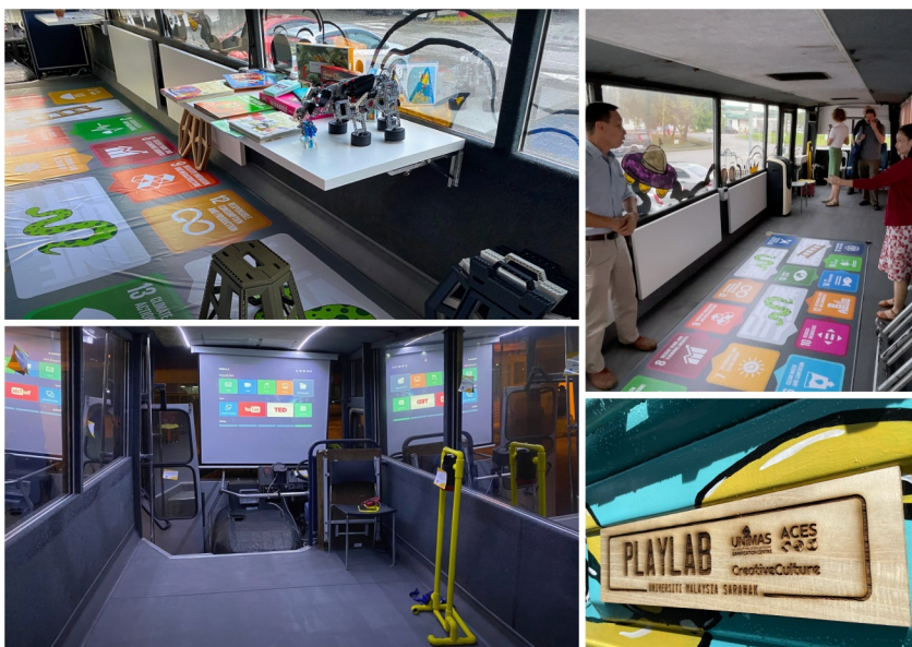
FIGURE 4 Example layout of the PlayLab Bus internal space, utilising hinged fold-away tables, concealed projection screens with mobile projectors, compact foldable chairs, privacy glass and energy efficient strip lighting.
