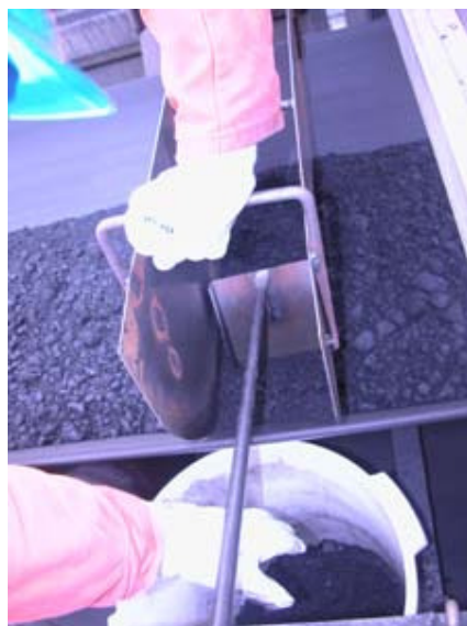
Figure 5. Stopped belt sampling results in structurally correct samples. Correct increment delineation and extraction is ensured in the above situation by using a device with fixed, parallel sides and a brush to extract all the fines along the bottom etc.
