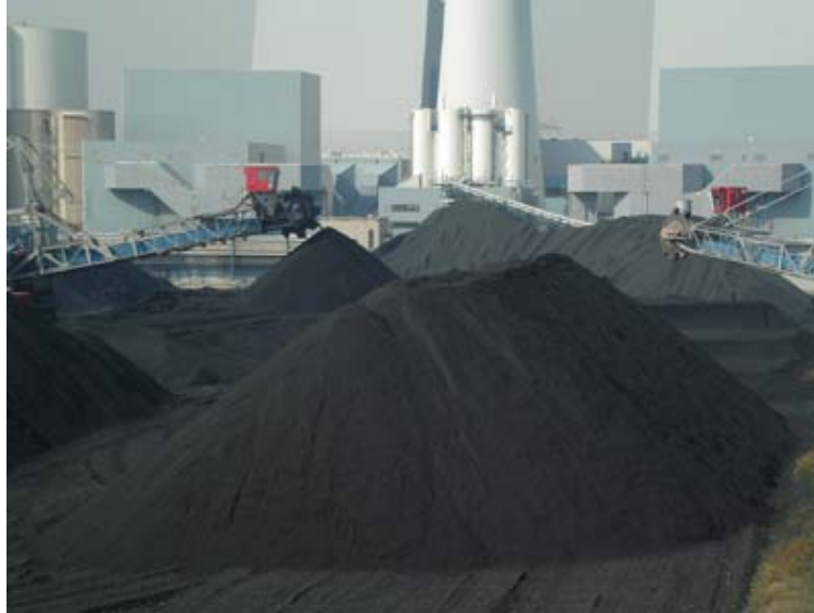
Figure 4. A large stockpile is for all practical purposes impossible to sample directly in any correct way without enormous, in practise prohibitive, amounts of time and effort. But no stockpile was ever born into this physical form directly however – on the contrary: it was certainly laid up incrementally , witness the various conveyor belts present. This simple fact opens up for another approach to completely correct and representative sampling! The example shown here is in point of fact scale-invariant , i.e. this pile can be envisaged at practically all scales.
