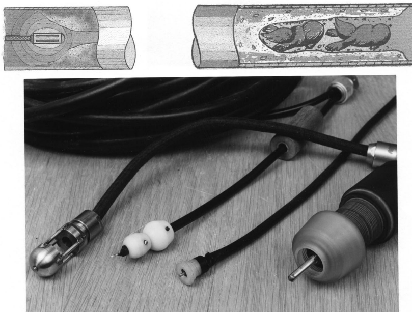
Fig. 3. Installation for cleaning of pipes from internal deposits
