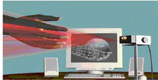
An illustration of a sensor tracking hand movement. The infra-red sensor (invisible light to the human eye) registers movement in its field. Here a hand enters the field and affects the dynamic feedback image (in this case a hand throwing a ball). Since the sensors track only movement other parts of the body (eg. trunk, leg) could just as well be controlling the feedback which in turn could be different (e.g. music, game etc.)
