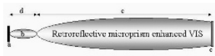
Figure 3: VIS enhancement technique (a) sensor head (b) beam dimension without enhancement (c) enhancement retroreflective material (d) approximately 1 meter (e) additional reversed polarity active space of around 12 meters plus.
