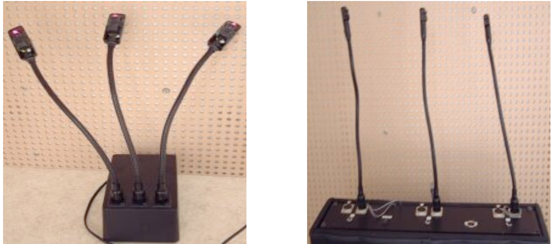
Figure 3: Three-head prototypes (c. 1993 left and c. 1999 right v ). The smaller sensor heads (on right prototype) are extendable via XLR cabling, which improves sensor location for operation (e.g. reaching over wheelchair arms/leg support), which augments user inclusion.
