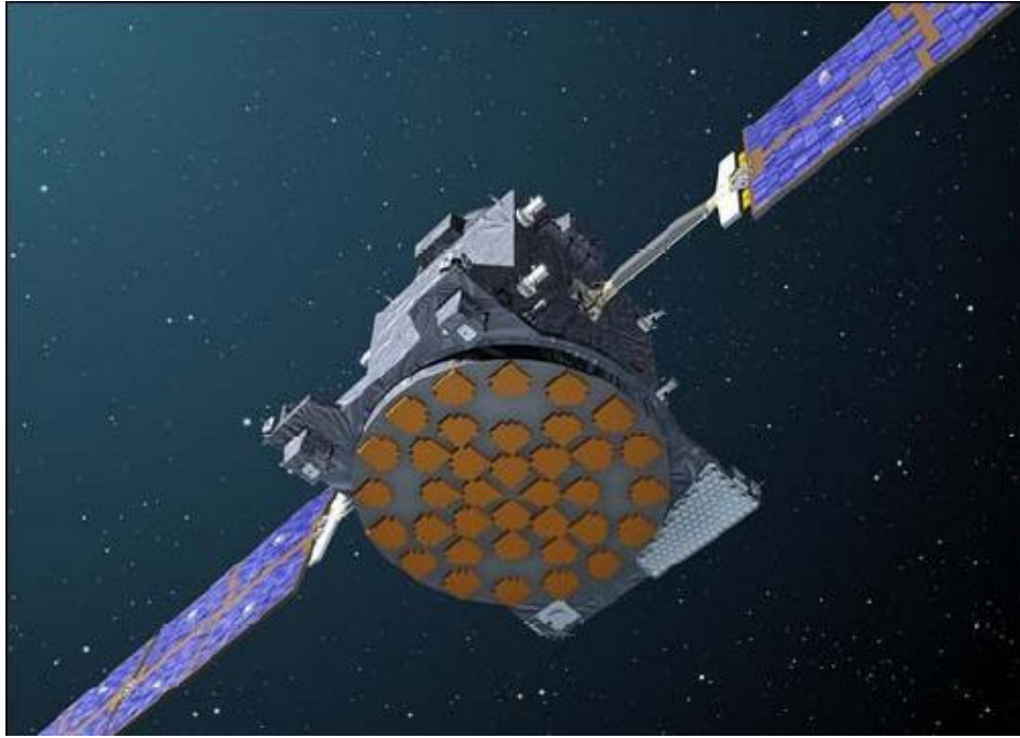
Fig. 1.1.4 Bottom view of a Galileo satellite showing the phased array antenna elements (courtesy: ESA)
