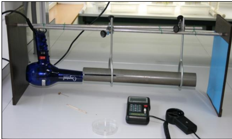
Picture 2. Wind tunnel designed to determine the role of the wind in achene dispersal.
