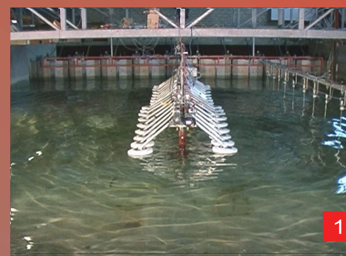
Figure 2: Wave tank Aalborg University. 1:40 scale Model tests. Subject to Torque T, mech. efficiency \eta & Power P_{out} analysis
