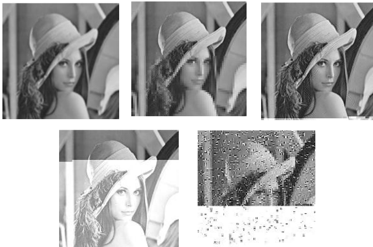
Figure 2. Images with image artifacts as follows: blurring, blocking, ringing, masking and lost blocks
