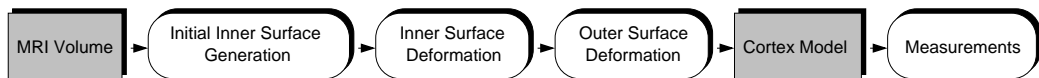
Figure 2.1: Pipeline of the method. Rounded boxes indicate processing steps. Gray boxes indicate data.
