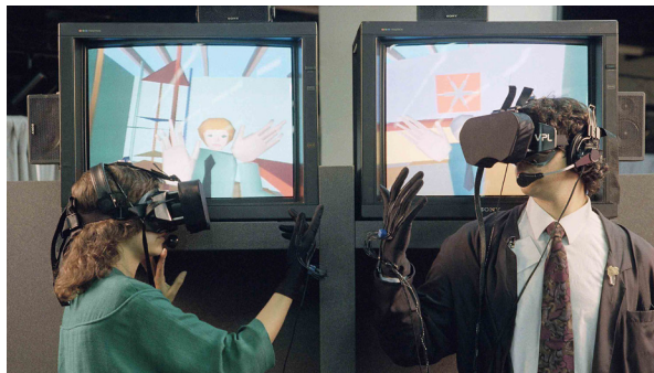
Two players immersed in the same virtual world (Reality Built for Two) with VPL Research's EyePhone headset and DataGlove. See database entry.
