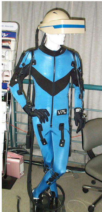
The DataSuit, created by VPL Research, measuring the movements of the entire body. See database entry.
