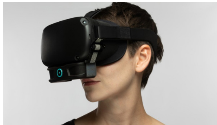
The INHALE VR headset by OVR Technology, which incorporates the sense of smell in the virtual reality experience. See database entry.
