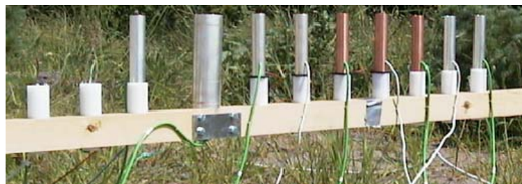
Figure 5. Experimental setup: testing of shielding techniques for air temperature measurements under direct solar access.
