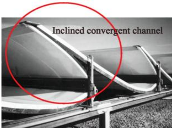
Fig. 2: Two experimental prototypes of the hydro-solar chimney that includes an inclined convergent channel.
