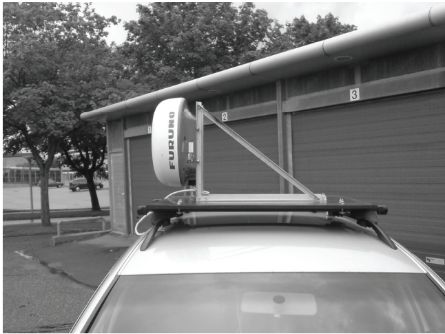
Fig. 2. The modified Furuno 1715 Microstrip Antenna mounted on top of a car.
