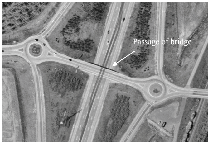
Fig. 8. Google Map© with GPS track overlay (both ways). The first loss of signal in Figure 7 is coinciding with passage beneath the bridge.
