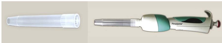
Fig. 9. Equipment used in evaluation of vial-to-Petri dish extraction. Left: “pseudo COLIWASA” (operated manually by thumb-pipetting). Right: cut, standard automated pipette. Note that both these alternatives allow for sampling of “sticky” material following [6].
