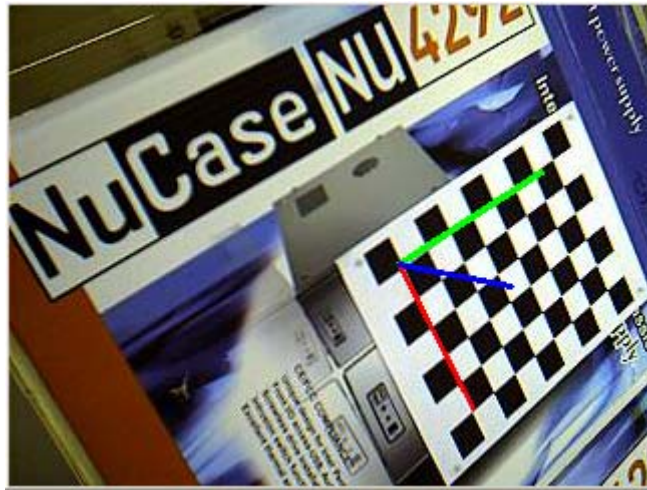
Figure C.2. shows the projection of the computed reference-frame.
