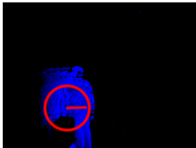
Figure 3.1.2 Motion History Image of the Figure 3.1.1., the circle with the line represent the direction and the location of the movement.
