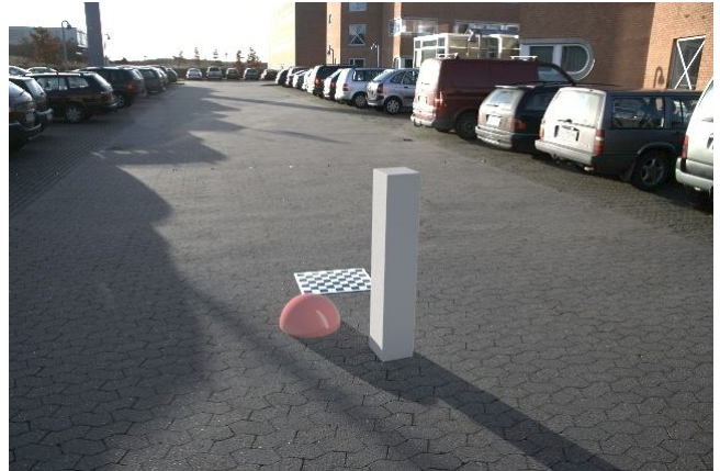
Figure 5: The checkered surface is used for calibrating the camera to the ground plane since we do not at present have an inertial sensor to provide the direction of gravity.
