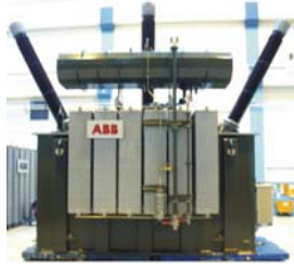
Fig. 4. 420 kV shunt reactor used for the cable/OHL line
