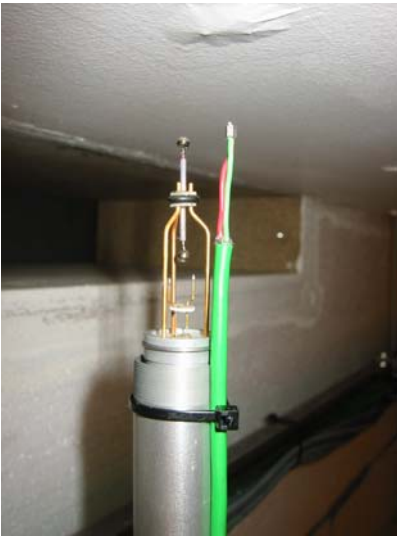
Figure 10. Anemometer and thermocouples for local air and ceiling surface temperature measurement.
