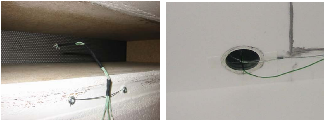
Figure 15. Thermocouples for measuring inlet (left) and outlet (right) temperatures during mixing ventilation.
