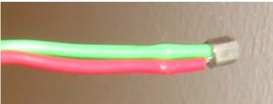
Figure 2. Thermocouple with aluminium tip.
