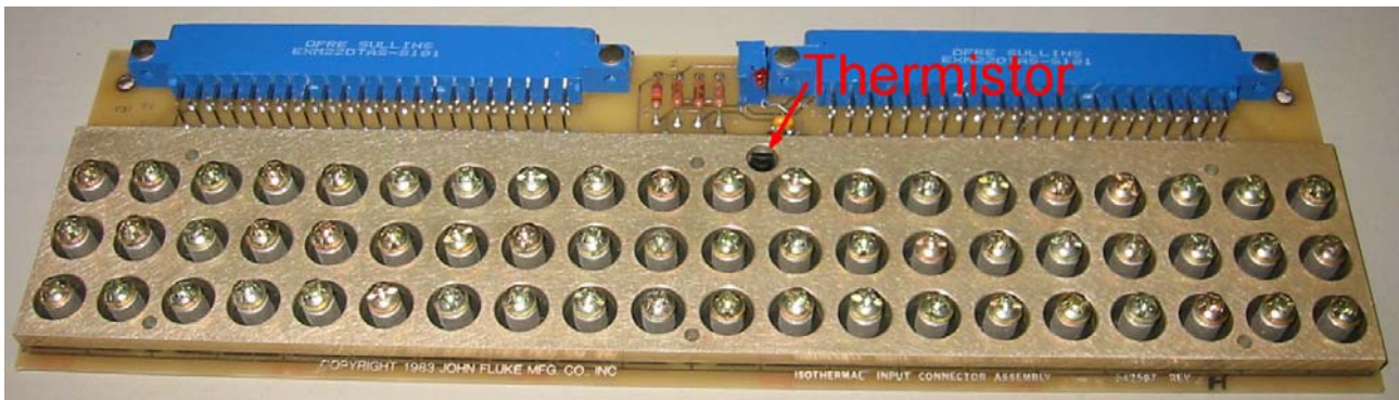
Figure 6. FLUKE Thermocouple/DCV Connector (175), cover removed to show the aluminium block and the thermistor.
