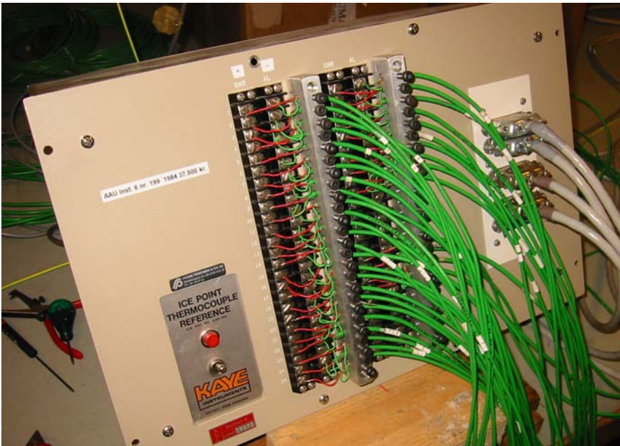
Figure 7. KAYE 170-50 ice point reference with 50 channels.
