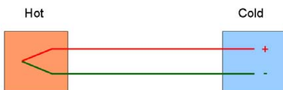
Figure 1. Functional principle of thermocouples
