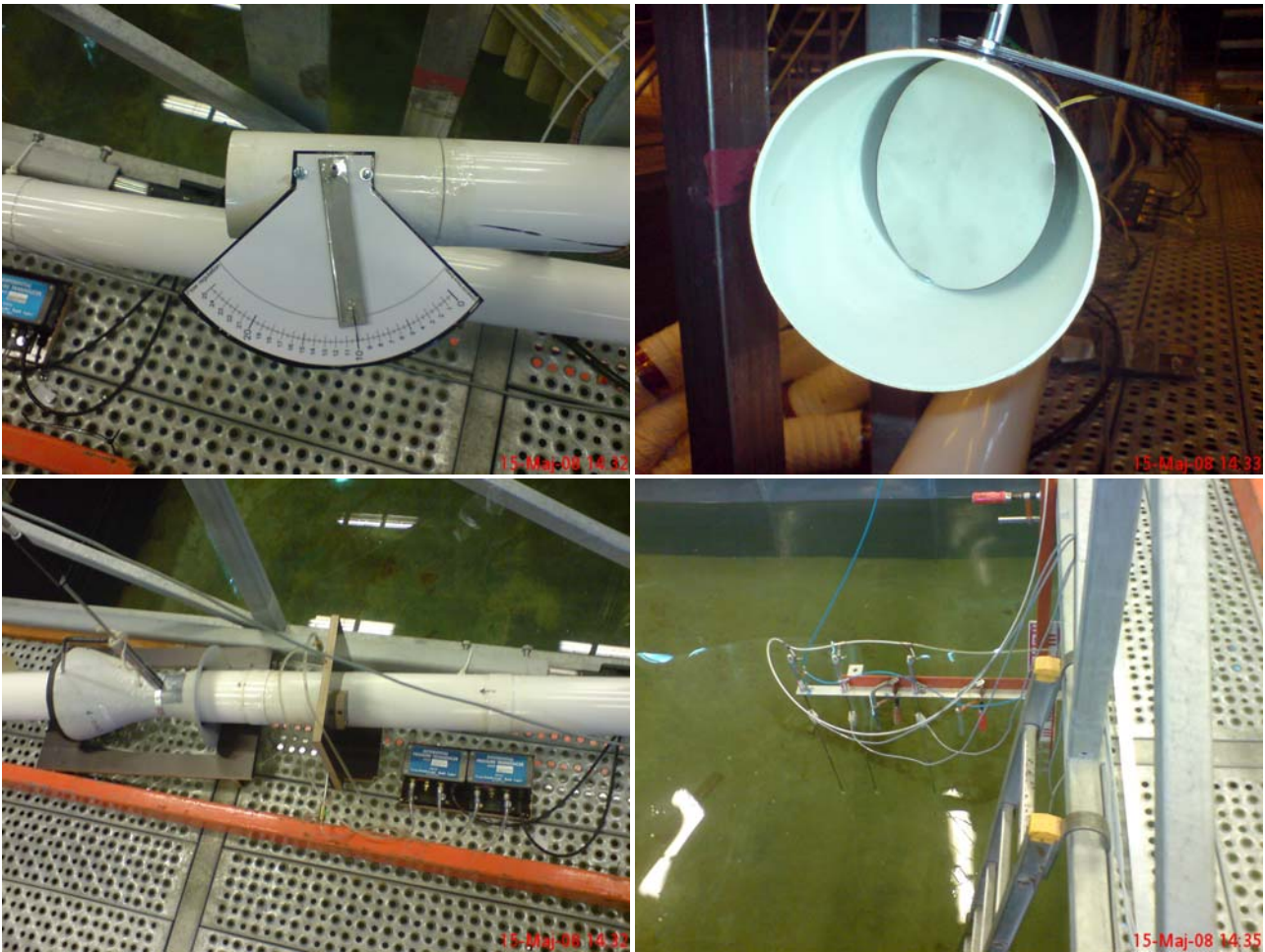
Figure 3 Upper: Valve and scale for valve for regulation of flow (corresponding to load on PTO) in intake. Similar setup used for exhaust. Lower, left: Thermo based flow speed measuring device placed in exhaust pipe. Lower, right; Wave gauges placed in front of right half of model, used for reflection analysis of waves.
