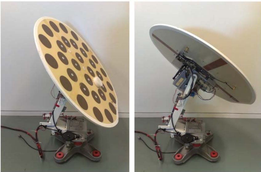
Figure 1.1: F77, SpaceCom's satellite tracking antenna.
