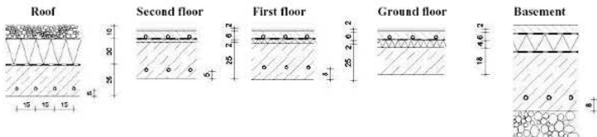
Figure 3.7 – Different positions of pipes as used in the ZUB in building Kassel, Germany (De Carli et al 2003)
