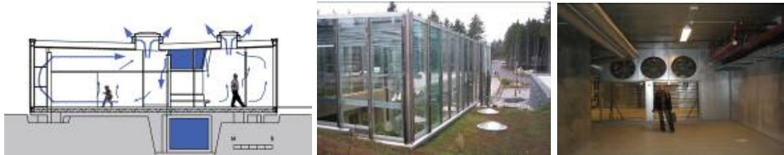
Section through pupils' base area, level 2. Ventilation air is led from the culvert via shafts to a distribution chamber over the secondary rooms ('spine'). The exhaust air is evacuated via the skylights (left). The air intake is through the glazed entrance of the building (middle), down to the underground culvert (right).
