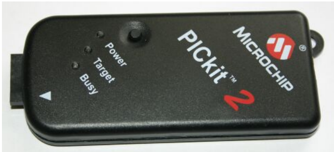
Fig. 3. A picture of the PICKit2 programmer that allows to program the opensensor.
