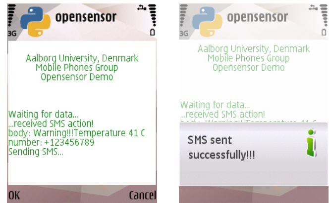
(a) The opensensor sends to the phone an SMS action command when the temperature exceeds a certain value. (b) The phone receives the SMS command and sends an SMS to a specified number.
