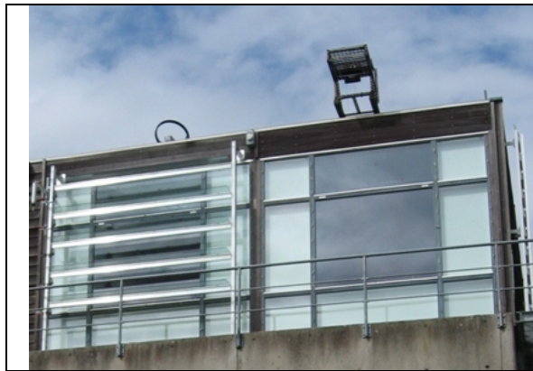
Figure 4. At left: glass lamella system in front of test room. At right: reference room.
