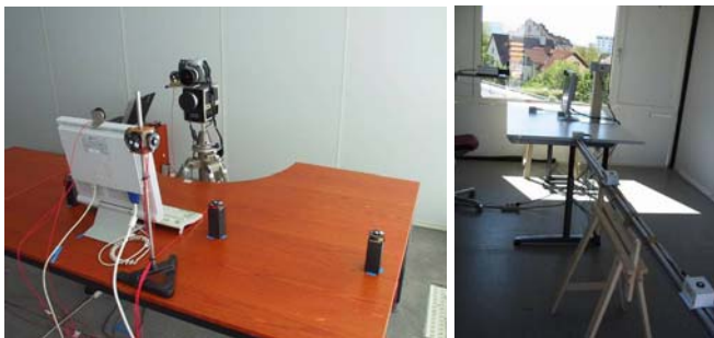
Figure 2. Interior view of the work place with CCD camera at eye position and interior illuminance sensors in the reference room (parallel view set up) at the SBi (left) and at ISE (right).
