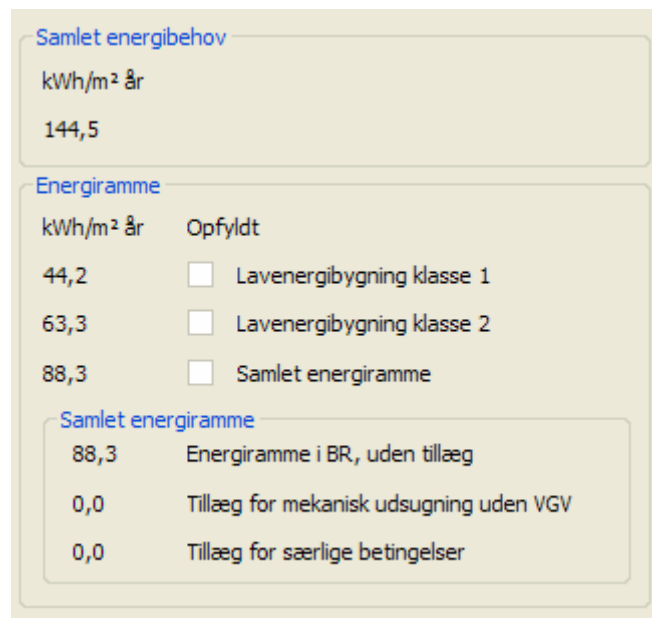
Figure 1. The energy frame calculations provided by Be06. Top - Total energy calculated consumption is 144.5 kWh/m 2 per year. Centre - The energy frame for this size of building is calculated to be 88.3 kWh/m 2 per year. To meet the requirements for low energy class 2 and 1 respectively, the calculated energy consumption must be below 63.3 kWh/m 2 per year and 44.2 kWh/m 2 per year respectively. At the middle of the screen are the energy frames for low-energy class 1 (44.2 kWh/m 2 per year), low-energy class 2 (63.3 kWh/m 2 per year), and the maximum energy frame for a new building according to the current building code (88.3 kWh/m 2 per year). Bottom - Resulting energy frame is shown in case of extensions of the energy frame due to special circumstances, of which there are none in this case.
