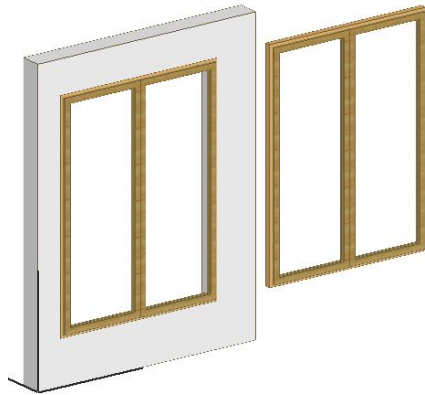
Figure 14: Window in Wall – Window replaces wall
