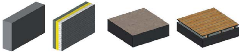
Figure 27 – Modelling of walls and floors gradually to greater detail
