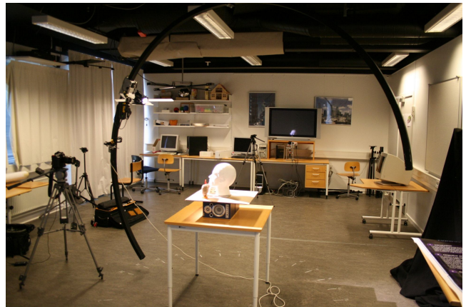
Figure 2: The actual sphere gantry on the lab. Unfortunately the rig is not motorized so it is manually moved during acquisition.
