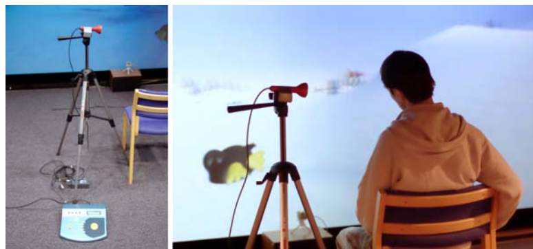
Figure 2. The SoundBeam device — a player steering the penguin with head movements.
