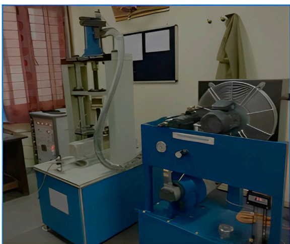
FIGURE 5 Fatigue test of the beam specimen.
