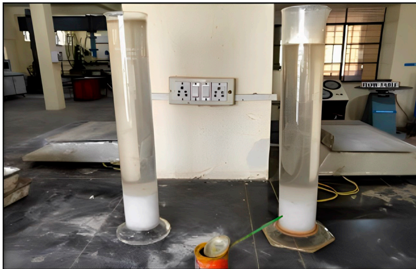
FIGURE 3 Preparation of alkaline solution from sodium hydroxide and silicate pellets.
