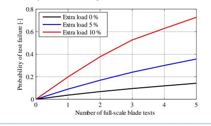
For both ultimate and fatigue limit states there is a decrease in the partial safety factor when additional full-scale tests are performed. If a extra load in the magnitude of 5 - 10 % is applied during testing it leads to a a significant decrease in the partial safety factor.
