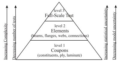
Normally several tests are performed with small coupons of the base material and a limited number of tests are performed with elements of the blade.
