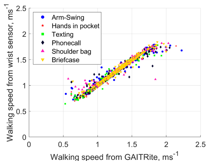
Figure 3. Relationship between wrist sensor and electronic walkway measured walking speed. N = 101 with 1487 walks. Each individual dot represents an individual data point. Combined data from six walking conditions.
