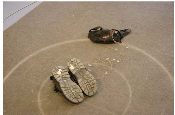
Figure 3. The sandals enhanced with pressure sensitive sensors wirelessly connected to a microprocessor.
