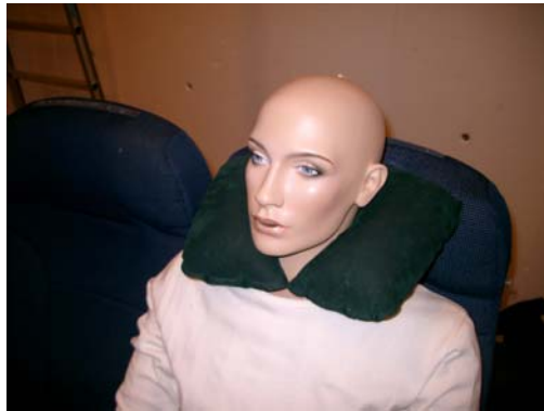
Figure 3. Manikin with a neck support pillow as a personalized ventilation device.
