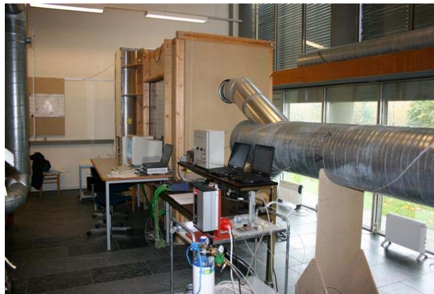
Figure 2. Wind tunnel for experiments with draught and personalized ventilation.
