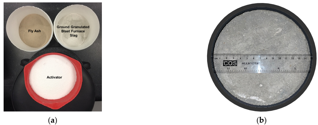
Figure 1. Geopolymer material: (a) binder and activator used for the production of the reference geopolymer material; and (b) produced reference sample.
