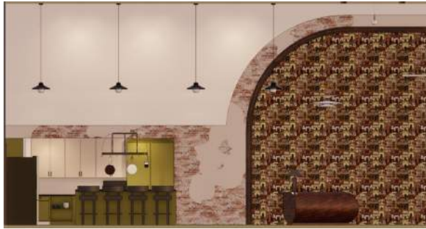
Figure 5.5 - Hostel south wall elevation which depicts original plastered brickwork, curves referencing facades, and salvaged flooring.
