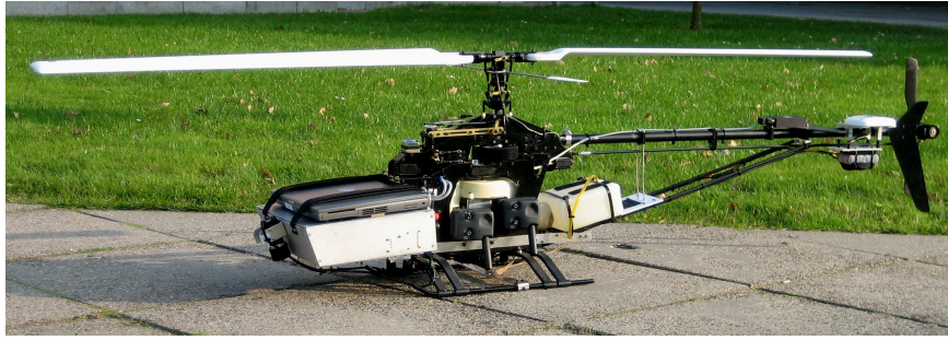
Figure 2.1: The modified Bergen Industrial Twin developed as test platform in this research.
