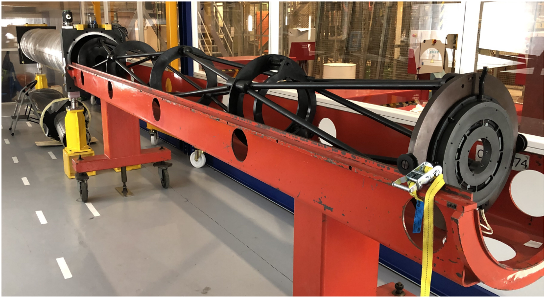
Figure 5. CEDAR-H under construction in a clean room at CERN. The photo shows the cylindrical gas vessel (silver-coloured part on the left of the image) and the support structure of the optical system (black part) sitting on a specialised CEDAR workbench (red part). The diaphragm can be seen at the end of the support structure on the right of the image.
